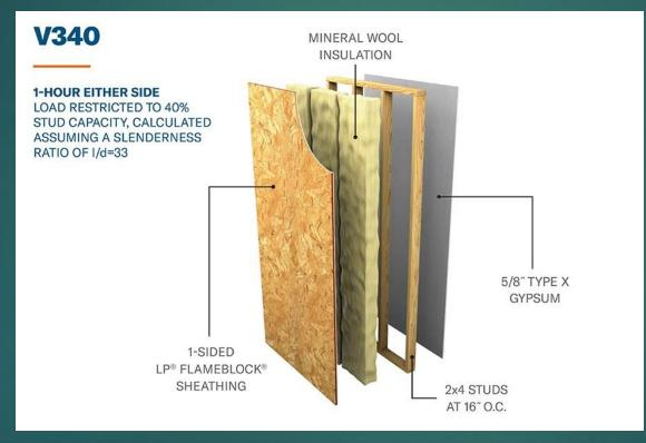
Fire-rated assemblies define a prescriptive list of materials used and the configuration of such materials. These include fire-retardant-treated lumber and/or plywood, gypsum board, insulation batts and blankets, and in some designs, fasteners.
