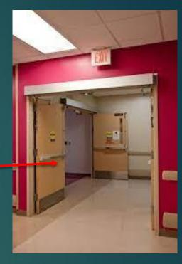
1910.36(a)(3)An opening into an exit must be protected by a self-closing fire door that remains closed or automatically closes in an emergency upon the sounding of a fire alarm or employee alarm system.
